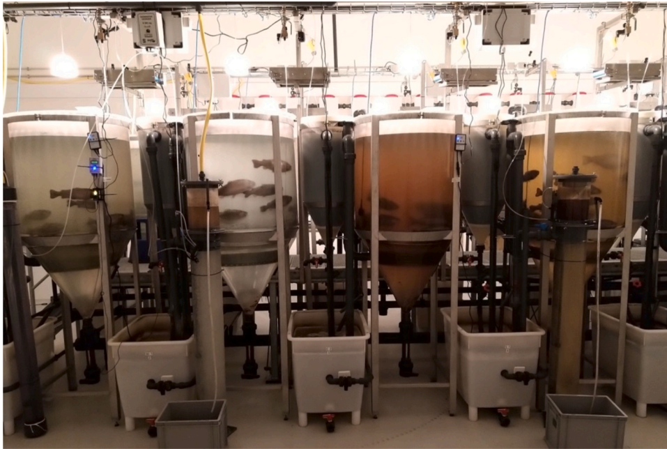
Fig. 3. Visible effects of the different treatments on water clarity. From left to right: Ozone, Ozone + foam fractionator, control and finally foam fractionator.
